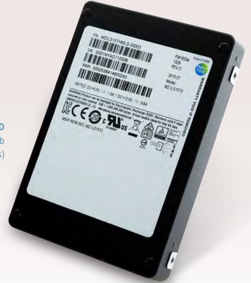
15.36TB SAS SSD (equipped with 512 of 256Gb V-NAND memory chips)
